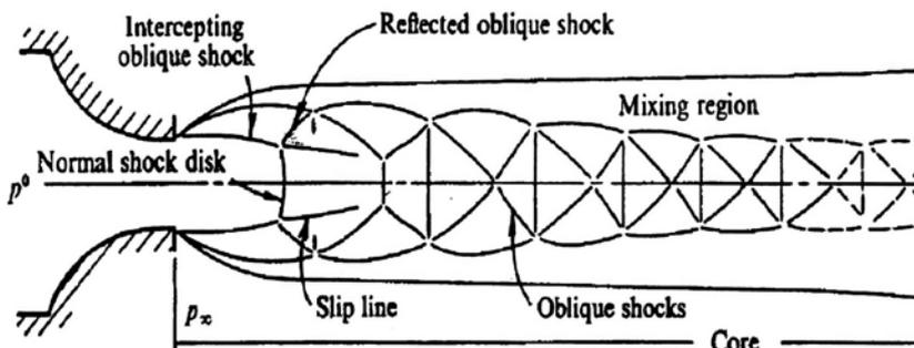
Figure 3. Air behaviour downstream of the nozzle: Near Field.
