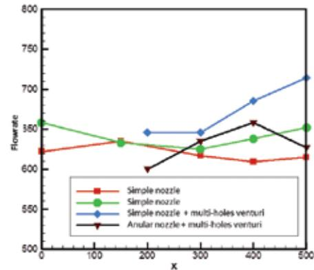
Figure 17. Comparison of mass flow rates [g/s] in laboratory tests.
