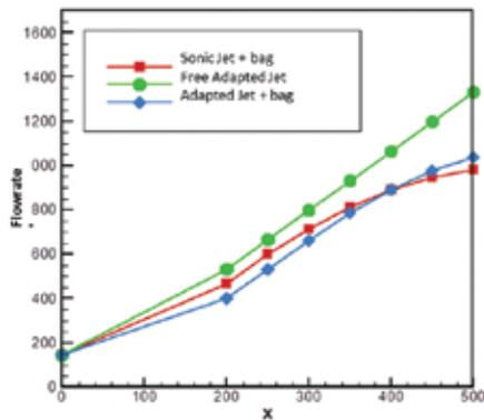
Figure 6. Mass flow rate [g/s] with different nozzles.
