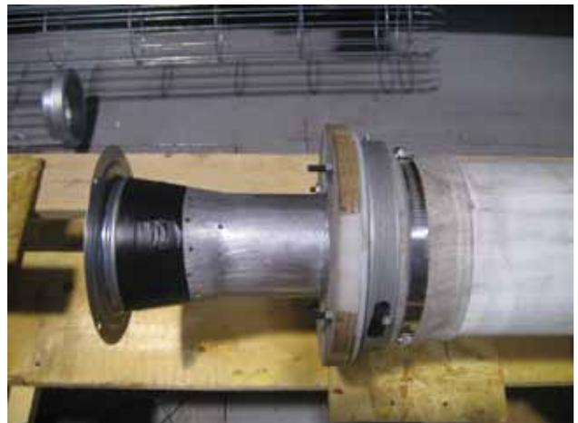
Figure 16. Venturi at bag inlet – holes system for air entrance.
