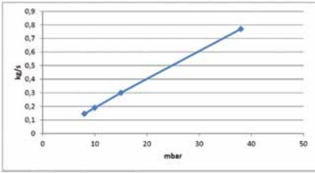
Figure 12. Correlation curve between pressure and flow rate inside bag.
