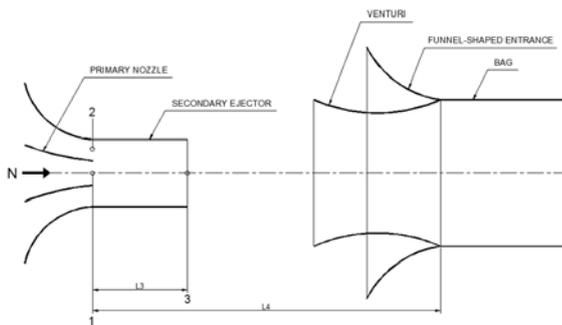
Figure 2. Geometry of the system.
