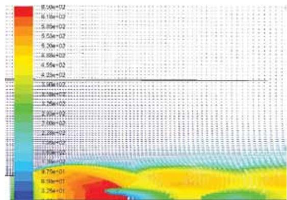
Figure 10. Air speed [m/s] at ejector outlet.
