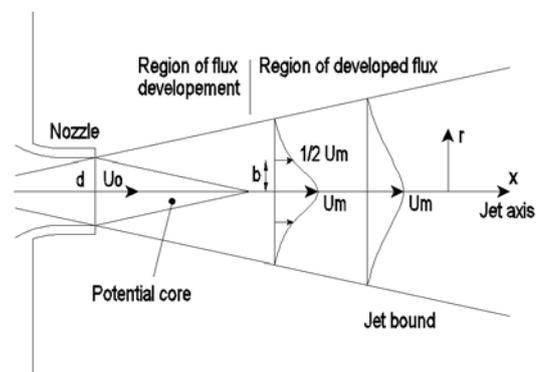
Figure 4. Air behaviour downstream of the nozzle: Far Field.
