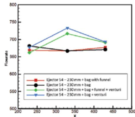
Figure 18. Direct comparison of flow rate with or without Venturi with multi-holes.
