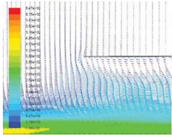
Figure 9. Air speed [m/s] at bag inlet.
