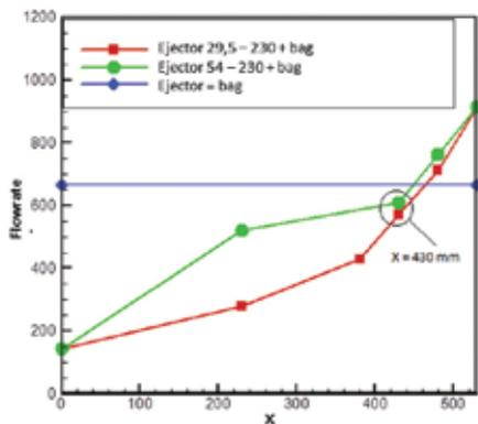
Figure 7. Mass flow rate [g/s] with secondary ejectors.
